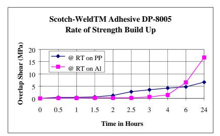
The above rate of strength build up was collected on 25mm\*100mm Aluminium and PP samples overlapped 12.5mm allowed to cure at 24°C and tested at a rate of 10mm/mn in overlap shear mode at 24°C.
