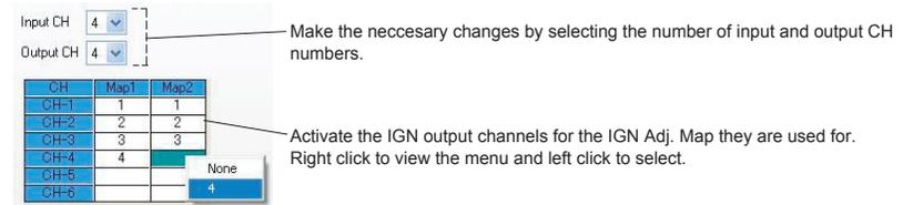
Make the necessary changes by selecting the number of input and output CH numbers.
