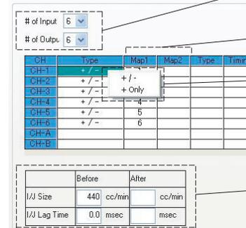
Set the number of Injector channels being used for main indicators.
