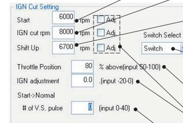
Input the start rev cut rpm. This will only activate only when e-manage does not detect vehicle speed signal and throttle position is above set value in "Throttle Position".
