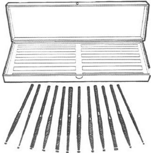
These files are usually supplied in sets. The most common set consists of twelve assorted files in a set which are marking (half-round), square, slitting, knife, joint (round edge), crossing (oval), barrette, flat, equaling, half-round, three-square (triangular), and round.
