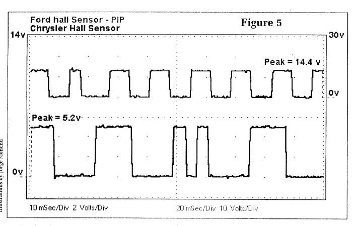
is often found at the top of the rising edge of the positive pulse. This signal characteristic does not seem to affect the performance of the circuit. In some cases it may have been intentionally placed there by the circuit designers.
