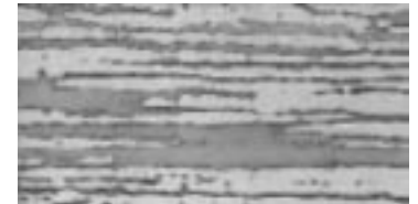
Duplex. (Austenitic-ferrite). Well-balanced two-phase structure with ferrite content between 30-50%.
