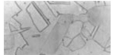
Austenite (γ-iron). Face centered cubic with 12 atom neighbours. 74% close packing.
