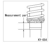
1. After installing the shock absorber on the vehicle, measure the area marked in the Figure, and adjust to match the reference values shown.
